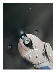
4. Tighten the lock nuts to secure the spider to the tube.
