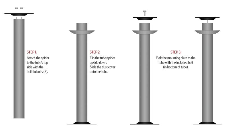
Bolt down bases should not be spaced more than 36" apart
