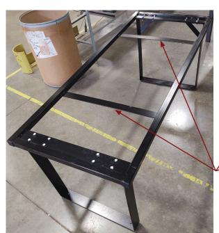
**Step 6:** Flip the frame with legs and glides attached to the top side up position.
