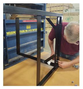
**Step 1:** On a clean, flat surface (such as a table topped with cardboard, place the top frame (D) on it's side.
