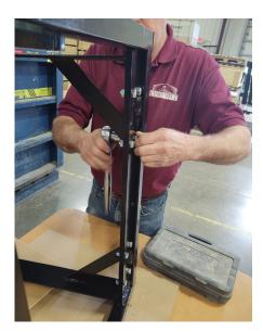
**Step 4:** Using a socket set and wrench, tighten all 8 bolts. *4 on each end.*
