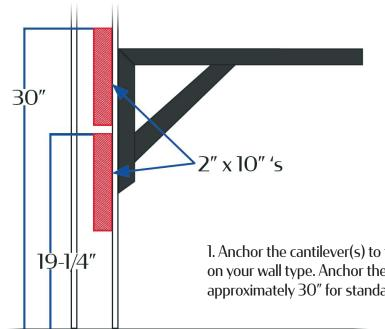
Please note, cantilevers should only be used on walls with appropriate support. Brick or masonry walls can be sufficient as long as specialty screws are used.
